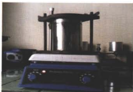
Fig. 1. Teflon-lined stainless steel autoclave (Hydrothermal method)
